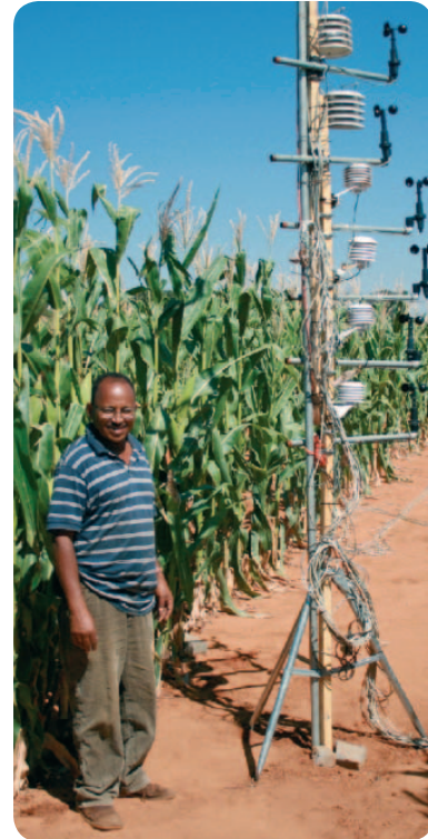
Mr Tesfuney Weldemichael, Ph.D. student, determining wind velocity with an anemometer in maize.
