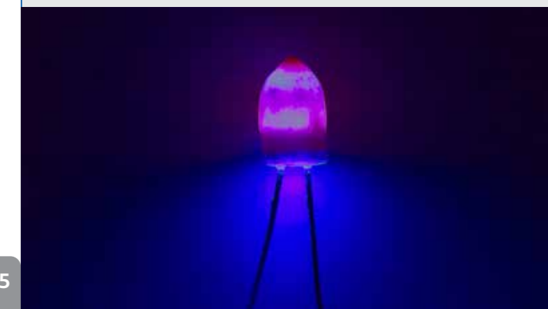
A strontium hexaborate (SrB 6 O 10 ) sample incorporated in glass to act as solar concentrators – from the research of Lucas Erasmus, a PhD student under the supervision of Prof Swart
