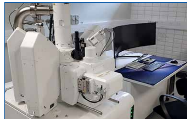
The newly acquired and commissioned EOL JXA-iSP100 Electron Probe Microanalyser (EPMA)
