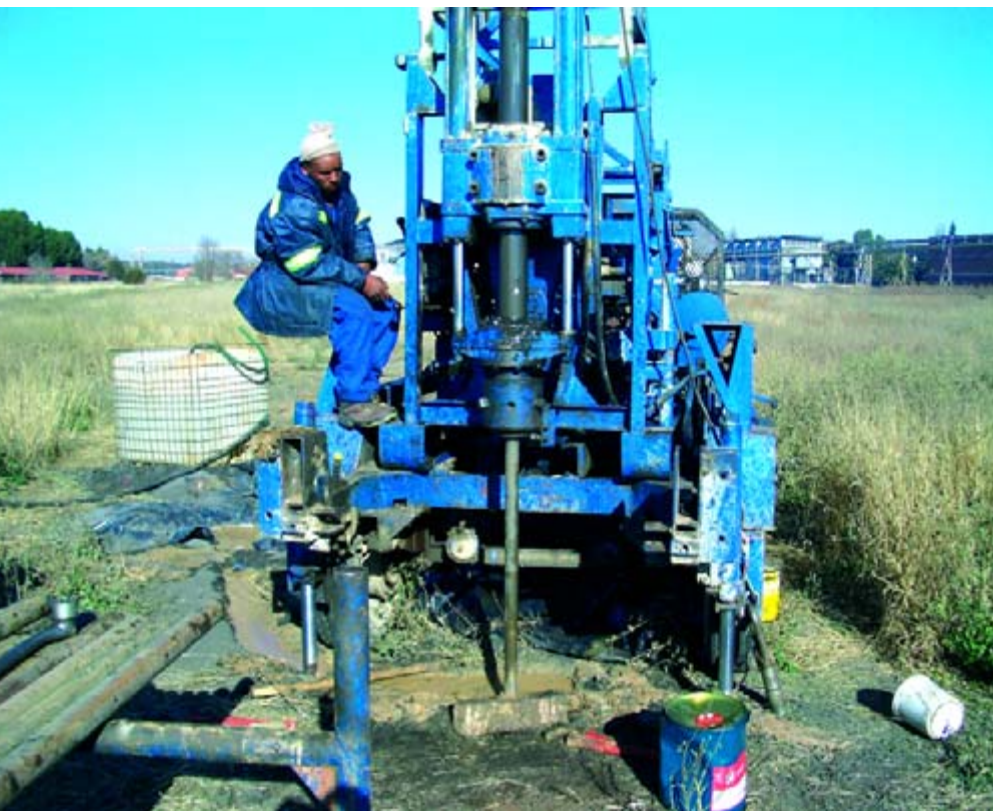
Drilling of additional core boreholes for the dense non-aqueous phase liquids in fractured rock research.
