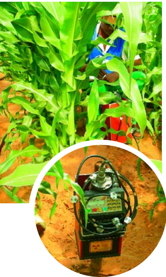
Lysimeter unit at Kenilworth Experimental Site for water and salt balance studies.
