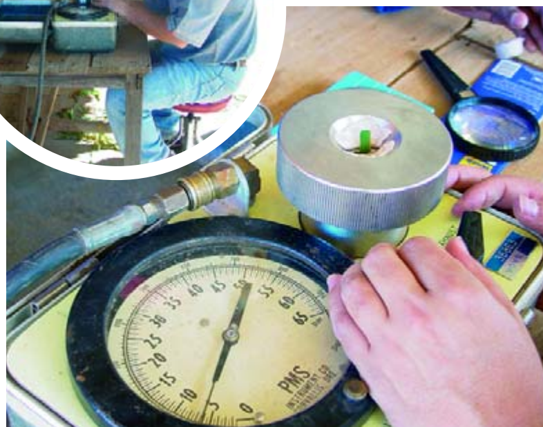
Prof. Leon van Rensburg, measuring the leaf xylem potential of irrigated maize using a Scholander pressure chamber. The leaf was sampled at the lysimeter complex of the Department of Soil, Crop and Climate Sciences at Kenilworth.
