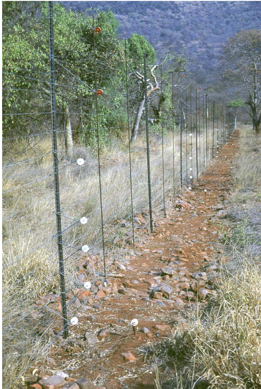
Figure 1 Electrified game fence with 21 smooth wires and nine electric wires used in the experiment.
