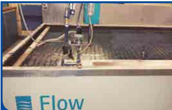
Flow water jet cutting stainless steel.
