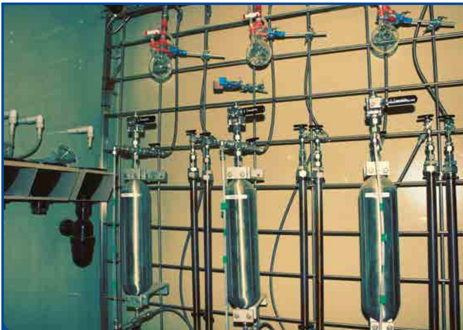
A dry-solvent percolator used to prepare dry solvents for organic reactions.
