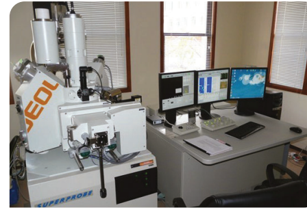
The Jeol JXA 8230 Superprobe at Rhodes University used by Justine Magson
