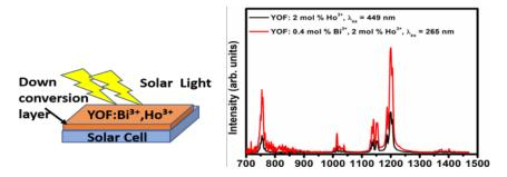
Illustration of the Down-conversion YOF:Bi<sup>3+</sup>,Ho<sup>3+</sup> layer on top of the solar cell, and the emission luminescence YOF:Bi<sup>3+</sup>,Ho<sup>3+</sup> phosphor.
