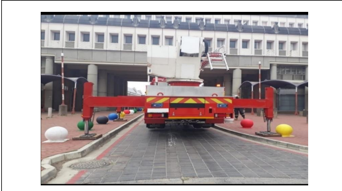
Figure 2.3 Aerial apparatus showing outrigger extended to support the aerial ladder (Aerial truck, Independence Avenue Bisho, May, 2019).
