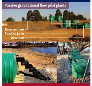
The BDAS system has demonstrated the capacity to remove up to 90 % of sulfate, 98 to 99% of iron and 90% of calcium in this system. The treatment is even effective in the removal of: Sr(92%) > Mg(22%) > K(8%) - Na(8%). The Ba values (0.1 mg/L) never exceed the limits of SANS drinking water standard (0.7 mg/L) while the EC and TDS decreased between 25 to 30%.
