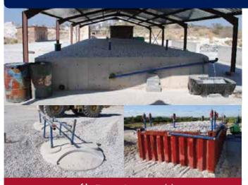
**Cr<sup>6+</sup> Pilot Scale Reactor(s)** Source Cr<sup>6+</sup> contamination: >5 mg/L >99% Cr<sup>6+</sup>removal (24hr HRT)
