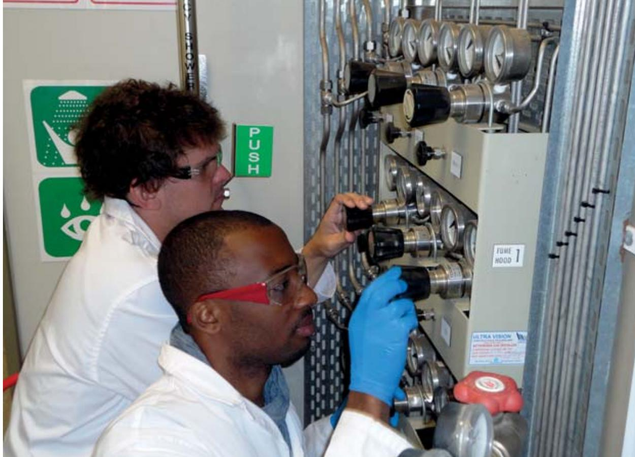
PhD student Renier Koen and MSc student Paul Bungu adjusting gases in the high-pressure autoclave reactor in the Homogeneous Catalysis Laboratory.
