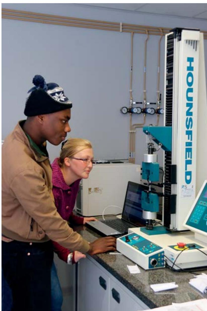
Two Polymer Science master's students, Chelley Clarke and Senzo Mdletshe, busy doing a tensile analysis on a polymer composite sample.
