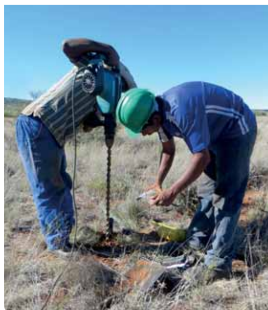
Preparing the soil to install DFM soil water sensor in the field at the Kolomela Mine near Postmasburg.
