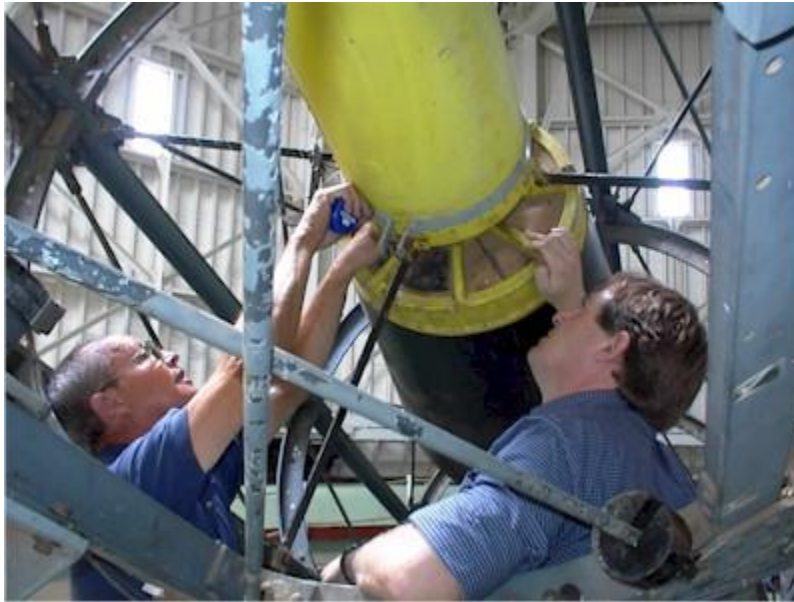
Ernie Fallows (technician) and Dr. Bill Craig (LLNL) investigate the focal distance on the secondary mirror of the 1.5-m telescope.
