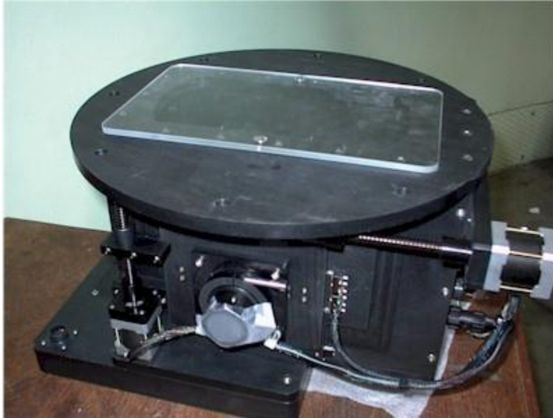
The acquisition box of the LLNL CCD camera system that contains the filter wheels and guide CCD camera.
