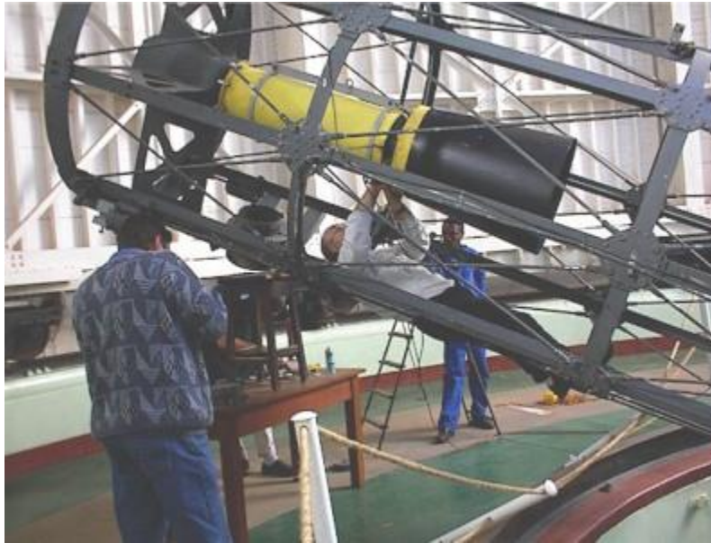
Frank Melsheimer working on the focus system, including a newly installed focus encoder, connected to the secondary mirror. Background: Simon Rakotsoana, technical assistant at Boyden Observatory.
