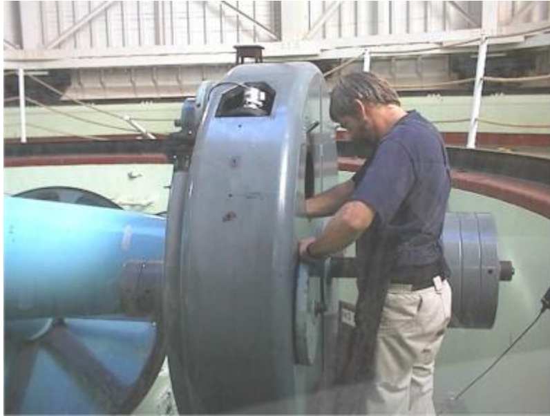
Ian working on the declination drive. The declination motor is visible through the opening on top.
