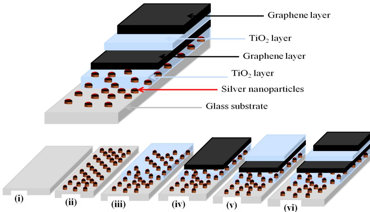
Figure 2: The schematic illustration for TiO<sub>2</sub> based plasmonic semiconducting thin film.
