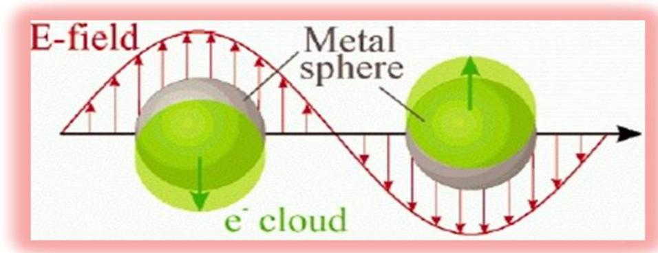
**Figure1: Localized surface plasmons on metal nanoparticles excited by free-space light.**
