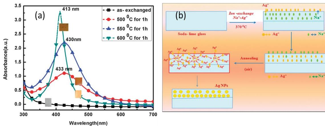
Figure 3: (a) : Optical absorption spectra with color photographs of the thermal evolution of Ag nanocomposite glass.;(b) : Thermal evolution of the Ag nanoclusters in an ion exchanged soda-lime glass
