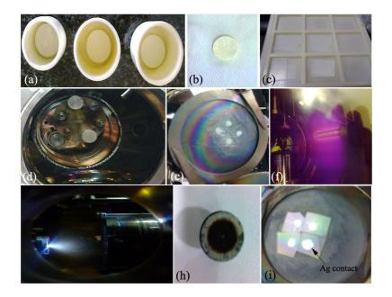
Photograph of various experimental procedures adopted in Pulsed Laser Deposition technique (a) pelletized ceramic target, (b) annealed target, (c), substrate cleaning, (d) target loading, (e) substrates loading, (f) removal of impurities in UHV chamber (glow discharge), (g) laser ablation, (h) ablated target, (i) as-deposited thin films.
